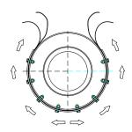
for open ended expansion joints with rectangular cross sections start from the corners. Spread out material equally between the fasteners
